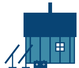
EQALUGAARSUIT Seqernup qinggorneranik katersiviit Panelit 180/67,5 kWp Batteriillu 167 kWh/100 kVA
