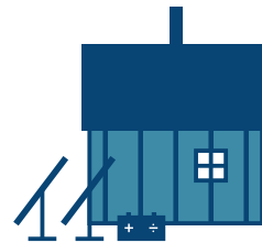
AMMASSIVIK Seqernup qinggorneranik katersiviit Panelit 102/33 kWp Batteriillu 167 Kwh/100 kVA
